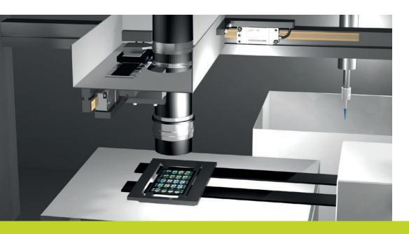
As an absolute encoder, the LIC 4100 provides the position value immediately upon switch-on without a reference run, ensuring high process reliability even in complex, long-running automated analyses. Reliability is further enhanced by signal processing from the encoder's built-in HEIDENHAIN Signal Processing ASIC (HSP 1.0), which eliminates the effects of contamination on the measuring standard. A functional safety option expands the encoders' range of possible applications.
