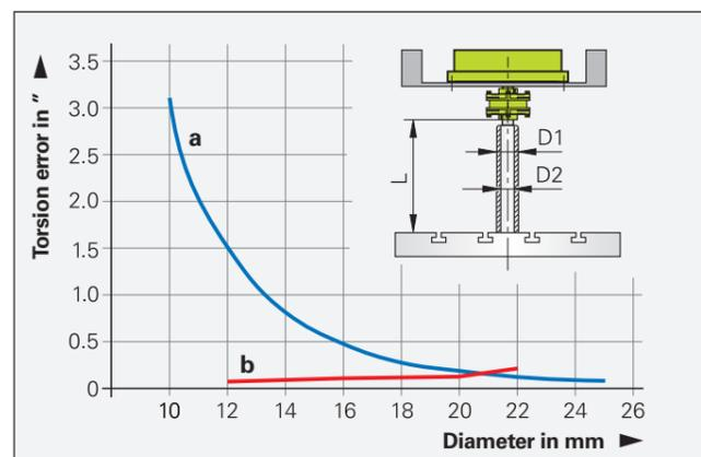
Torsion error of the 100-mm long coupling of an ROD 880 via a
