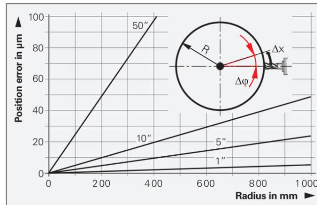
Influence of the distance R of the machining position from the center of the rotary table on the positioning accuracy  $\Delta x$  at various angular errors  $\Delta \varphi$  of the rotary table
